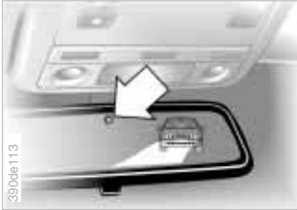
The semisolid reacts chemically to this electrical current, thus providing infinitely-variable dimming of the mirror (electrochromic technology).
