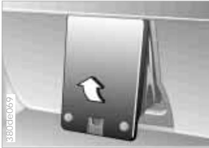
From the inside of the luggage compartment, use the magnetic retainers to attach the cover panel to the underside of the rear parcel tray.
