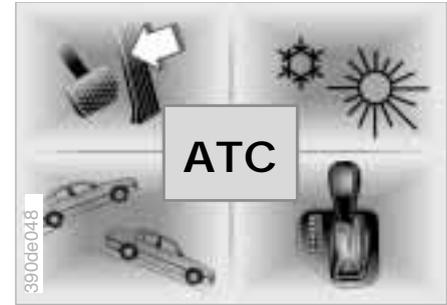
On vehicles with automatic transmission Adaptive Transmission Control (ATC) uses a number of factors to calculate the maximally efficient gear. In this process it monitors your personal driving style, the situation in which you are driving, the condition of the road and the traffic conditions.
