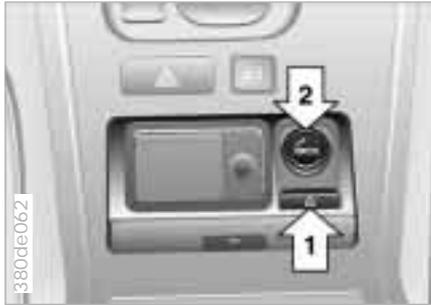
Push the lighter in (arrow 2). Remove as soon as the lighter jumps back out.
