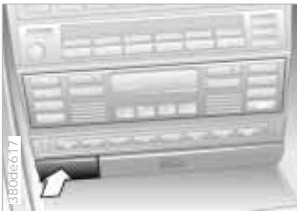
The interface socket for the onboard diagnosis system is located beneath a cover on the center console front panel (arrow).
