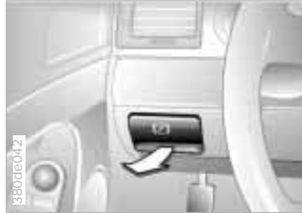
To release the brake, pull the handle. Please remember that the brakes disengage immediately. The parking brake is primarily designed to prevent the vehicle from rolling while parked, and operates against the rear wheels.
