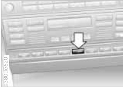
The system automatically ensures damping of the running gear on demand and thus increases comfort and driving safety.
