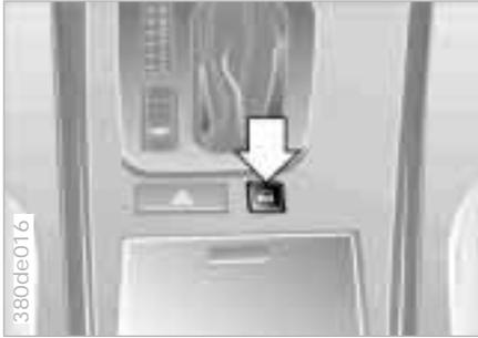
Use this button to operate the central locking system when the front doors are closed. With this button, only the doors and luggage compartment lid are unlocked or locked. The anti-theft system is not activated.
