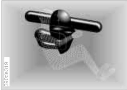
Deceleration sensors continuously monitor the physical forces acting upon the vehicle. In a severe frontal collision, the gas generators of the driver's airbag and the front passenger airbag are ignited. However, the passenger-side airbag is only triggered if an additional sensor has recognized that the passenger seat is occupied.
