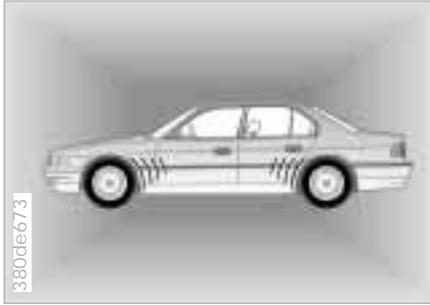
Near every wheel, there are antennas in the body which receive the signals from all four wheels. A central electronics system evaluates the quadruple signals which it receives and forwards any changes.
