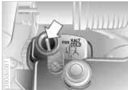
Correct coolant level when the engine is cold (approx. 68°F / 20°C):
