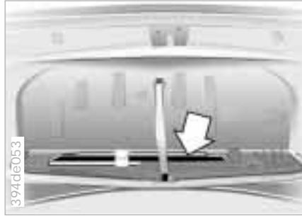
The hazard warning triangle is stored underneath the luggage compartment lid in the onboard tool holder where it is quickly available.
